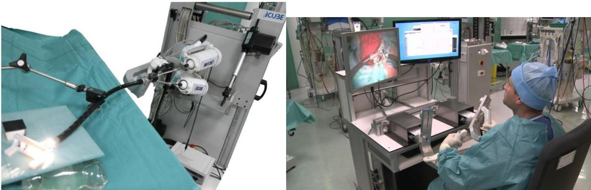
Fig. 1. left: Slave part of the STRAS platform. Right: Telemanipulation during in vivo trials.
